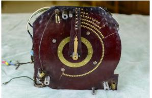
After a very careful inspection, I found several small things that needed fixing. The flat spring that returns the credit dial on the stepper unit, above the mechanism, was broke. A few wires were loose or badly frayed.
