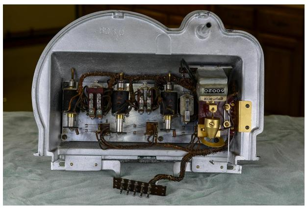
The back bonnet has several solenoids and relays plus a tilt mechanism and small mechanical counter attached. Sticking through the back bonnet is a reset button. All of the electrical "stuff" on the mechanism and the back bonnet plug into a stepper unit that sits above the mechanism. This stepper unit keeps track of winning combinations on the reels and shows the credits on the front.
